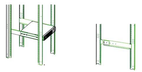
Adjust the rail according to depth of the rack. It should not be greater than the maximum size of the rack rail, and not be shorter than the minimum size of the rack rail as well. Fasten the rails with screws.
